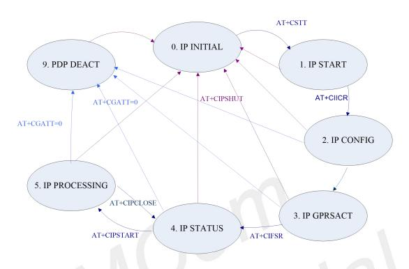
Figure3: APPTCP States Diagram for multi connection
